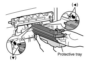
8 Install the waste toner cartridge (1) and slide the lock lever to the left (2).
